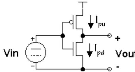
Steady state reached when  $V_{out}$  reaches value where  $I_{pu} = I_{pd}$ .
