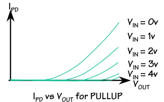
Nfets turn off when  $V_{GS}$  falls below the threshold voltage  $V_{TH}$ . So, even if the input voltage is, say, 5V, then the pullup will turn off when  $V_{OUT}$  reaches  $5V - V_{TH} = 4.2V$ . The pulldown will also turn off before  $V_{OUT}$  reaches 0V.
