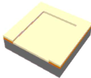
2. Then cover the whole chip surface with a thin insulating oxide layer.
