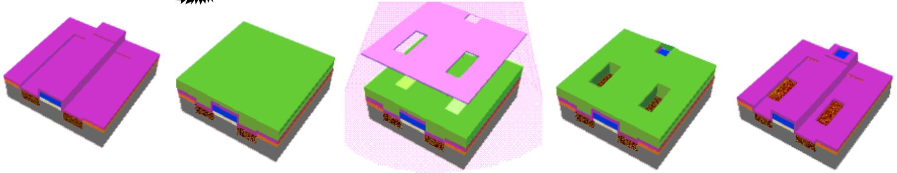
Each level of metal interconnect proceeds in two major steps. The first, shown in the sequence above, deposits an insulating layer of  $\text{SiO}_2$  and forms vias (holes) in the oxide to the layer(s) below. In this example, vias are made to the source/drain diffusions and the polysilicon gate.
