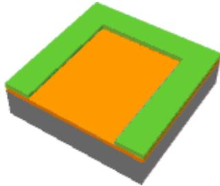
The exposed photoresist is removed with a solvent. The unexposed photoresist remains, masking portions of the underlying  $\text{SiO}_2$  layer.
