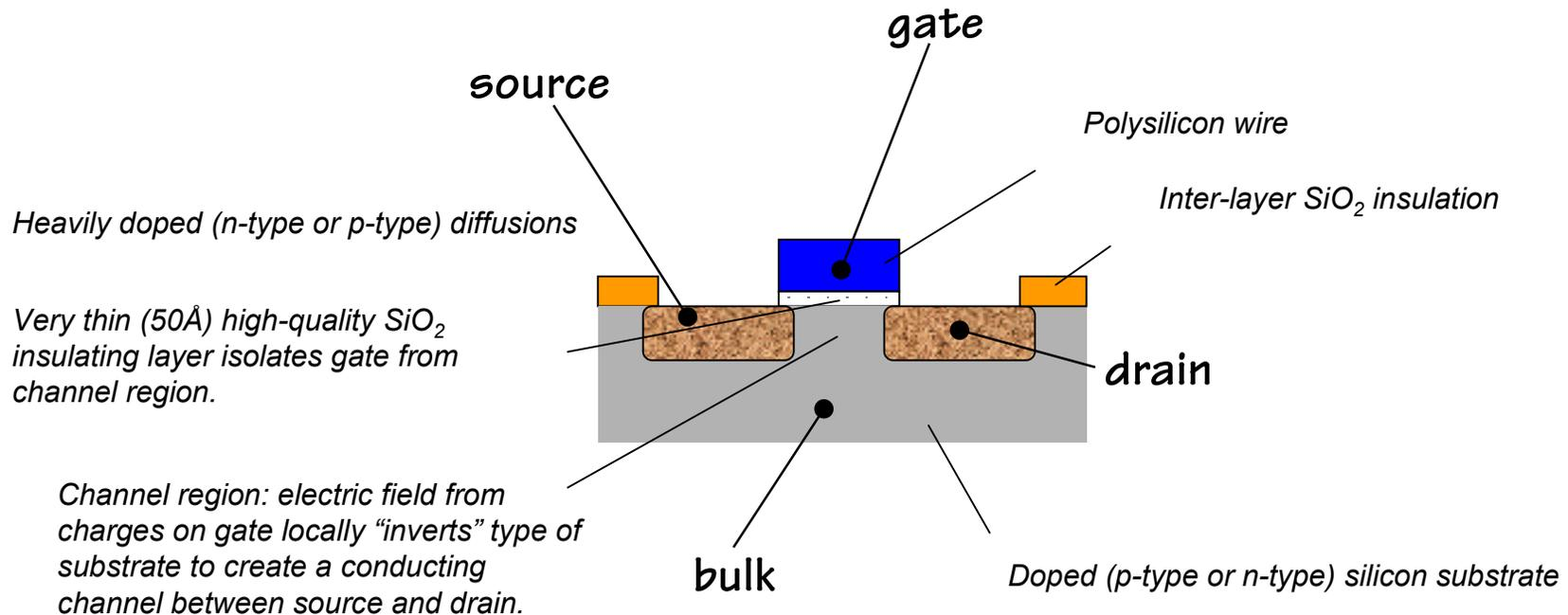
MOSFETs (metal-oxide-semiconductor field-effect transistors) are four-terminal voltage-controlled switches. Current flows between the diffusion terminals if the voltage on the gate terminal is large enough to create a conducting "channel", otherwise the mosfet is off and the diffusion terminals are not connected.
