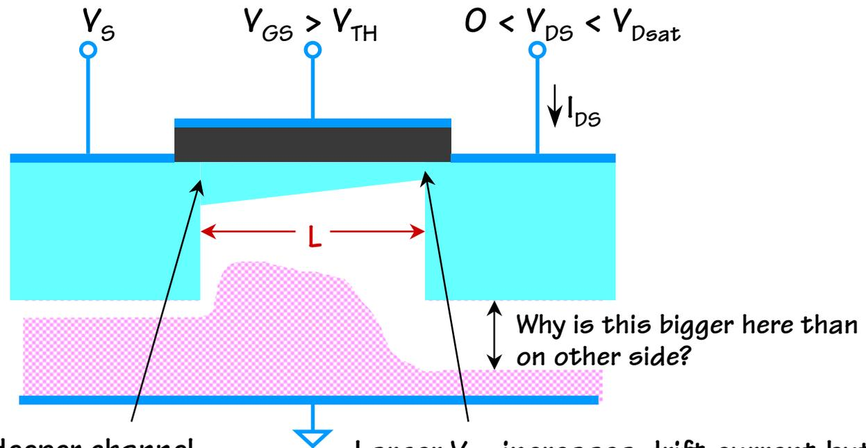
Larger  $V_{GS}$  creates deeper channel which increases  $I_{DS}$
