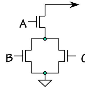
Step 2. Walk the hierarchy replacing nfets with pfets, series subnets with parallel subnets, and parallel subnets with series subnets
