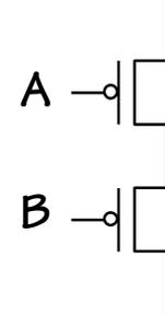
conducts when A is high or B is high:  $A + B$
