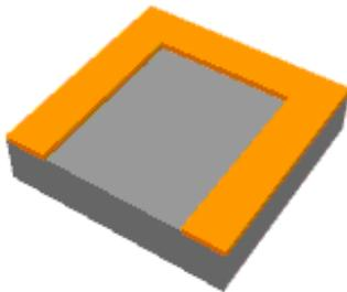
Finally, the remaining photoresist is removed with a different solvent and we're left with pattern of insulating  $\text{SiO}_2$  on top of exposed p-type substrate.
