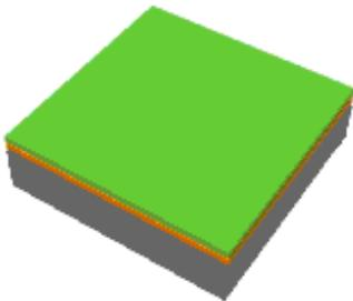
Now we’ll form a pattern in the  $\text{SiO}_2$  using a mask & etch process. First the wafer is coated with a layer of **photoresist**. Photoresist becomes soluble when exposed to ultraviolet light...
