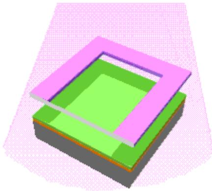
Using a **mask** to protect parts of the wafer, we’ll expose those portions of the wafer where we want to remove the photoresist. We’ll use different masks when creating each of the different structures on the wafer.
