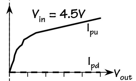
When both fets are saturated, small changes in  $V_{in}$  produce large changes in  $V_{out}$
