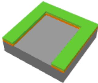
A chemical etch is then used to remove the revealed silicon dioxide.
