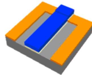
7. Remove the photoresist.
