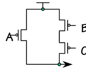
Step 3. Combine pMOS pullup network from Step 2 with nMOS pulldown network from Step 1 to form fully-complementary CMOS gate.
