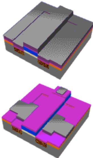
In the second major step, shown to the left, the aluminum is deposited, patterned, then etched to form low-resistance ( $.07 \Omega/\text{sq}$ ) interconnect. With planarization (a mechanical polishing step that creates a flat surface), multiple levels of metal interconnect are possible -- 3 to 6 layers are common in today's processes.
