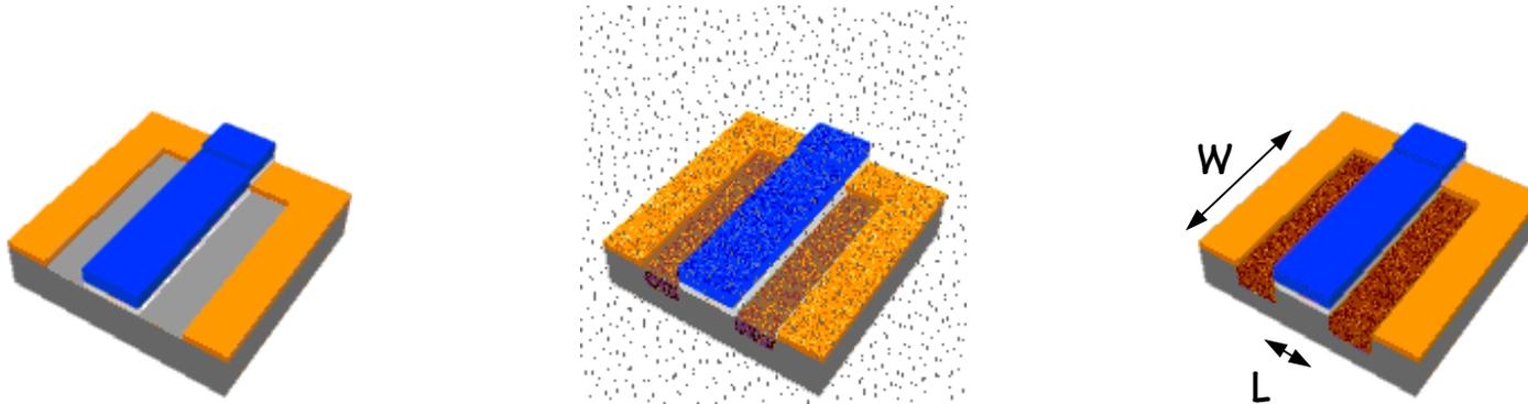
Donor implants are used to create **self-aligned** MOSFET **source/drain diffusions** and substrate contacts. Usually As is preferred to obtain shallow **N-type** diffusions and minimal lateral diffusion. High doses are needed to make low resistance ( $25 \Omega/\text{sq}$ ) diffusion wires. Afterwards a short thermal annealing step is performed to repair surface damage caused by the implantation.
