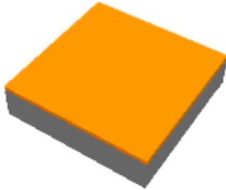
A “thick” (0.4 $\mu$ ) layer of  $\text{SiO}_2$  is formed by oxidizing the surface of the wafer with wet oxygen (we rust it!). The  $\text{SiO}_2$  will serve as insulation between the conductive substrate and subsequent conductive layers we’ll build on top of the oxide.
