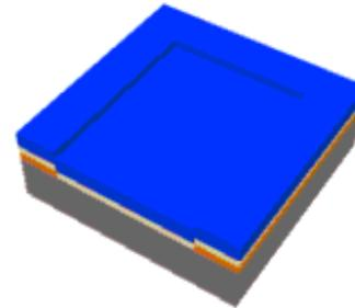
3. Cover that surface with a conducting "gate" material.
