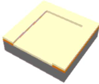
Now a “thin” (100 Å) layer of  $\text{SiO}_2$ , called **gate oxide**, is grown on the surface. The gate oxide needs to be of high quality: uniform thickness, no defects! The thinner the oxide, the more oomph the FET will have (we’ll see why soon) but the harder it is to make it defect-free. Coming soon to a fab near you: 50 Å gate oxide...
